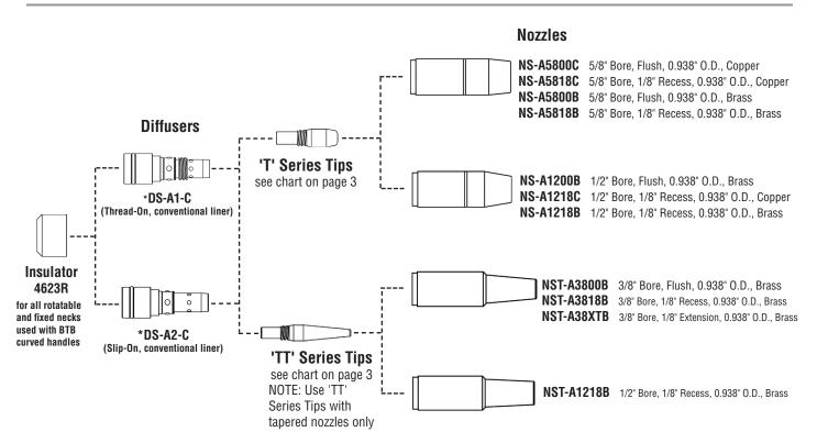
NOTE: \*Not engineered for error-proof liner replacement and flawless wire feeding. For use with Bernard conventional liners. Refer to spec sheet <u>SP-L</u> for more information.
