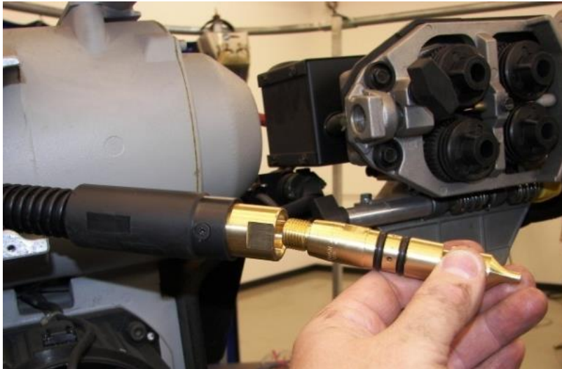
Figure 9 – Once the LSR uncable is pulled through the robot, add the power pin (or Euro connector).
