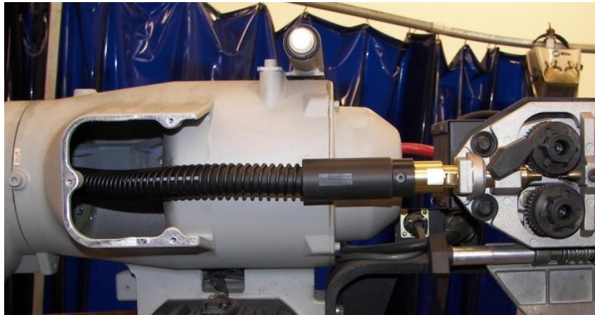
Figure 11 – Install the power pin or Euro connector to the wire feeder as per the manufacturer's instructions. The wire feeder control cable is also added during this step.
