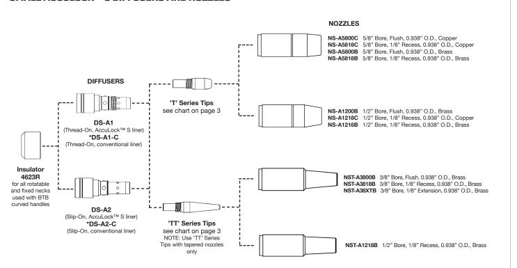
NOTE: \*NOT ENGINEERED FOR ERROR-PROOF LINER REPLACEMENT AND FLAWLESS WIRE FEEDING. FOR USE WITH BERNARD CONVENTIONAL LINERS. REFER TO SPEC SHEET SP-L FOR MORE INFORMATION.
