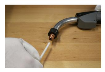
3. Lock and center liner by reinstalling the diffuser. Slide power pin cap over exposed liner and tighten the cap snug against power pin shoulder with welding pliers or appropriate wrench.
