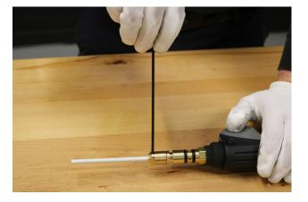
7. Insert a piece of welding wire into the liner to check for burrs or obstructions. If needed, loosen screw slightly until wire slides freely.
