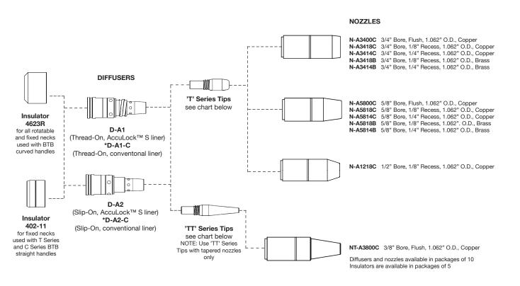
NOTE: \*NOT ENGINEERED FOR ERROR-PROOF LINER REPLACEMENT AND FLAWLESS WIRE FEEDING. FOR USE WITH BERNARD CONVENTIONAL LINERS. REFER TO SPEC SHEET SP-L FOR MORE INFORMATION.
