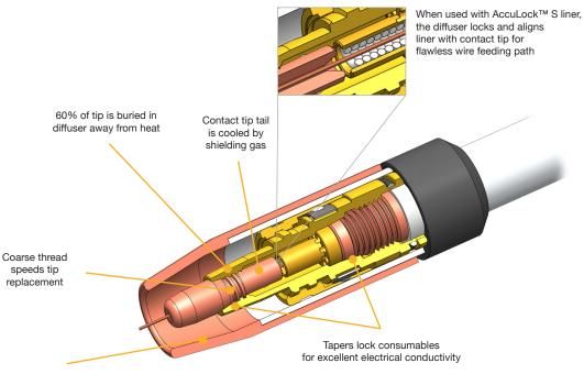
Nozzle stays in place during use / cleaning due to the steel retaining ring on the diffuser that helps to keep the threaded nozzle from loosening
