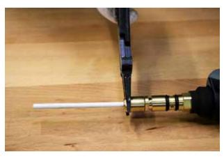
4. Holding a hex wrench as shown, tighten the screw "finger-tight" against the liner.
