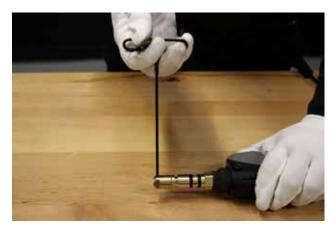
2. Replace the new liner through the neck until brass liner lock bottoms on neck.
