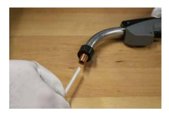
3. Lock and center liner by reinstalling the diffuser. Slide power pin cap over exposed liner and tighten the cap snug against power pin shoulder with welding pliers or appropriate wrench.
